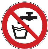
P005 - Eau non potable
